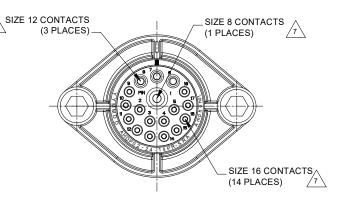
REDUCED DIA. WIRE SEAL SEALED PANEL MOUNT
