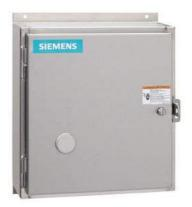
Mechanically held lighting contactor, Contactor amp rating 20Amp 0NC - 10NO poles, 208-240V 50/60HZ coil, Non-combination type, Encl NEMA type 4X 304 S-steel Water/dust tight noncorrosive
