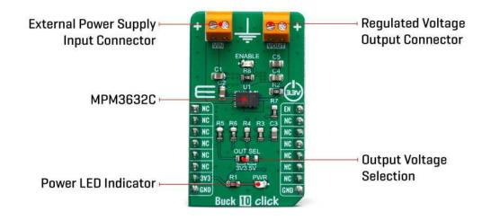
The output voltage is determined by the feedback voltage on the FB pin. Buck 10 click is equipped with a voltage divider and an SMD jumper, labeled as OUT SEL. This jumper can be used to connect one of two available voltage divider resistors, allowing the output to be set to either 3.3V or 5V. These two voltages are the most commonly used in embedded development.
