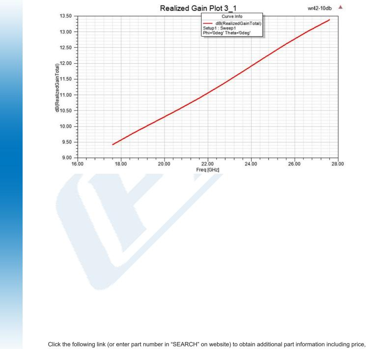
inventory and certifications: WR-42 Standard Gain Horn with 10 dBi gain, 2.92mm Male connector PEWAN042-10KM
