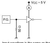
Input waveform is the same as that in case of switching characteristics test.
