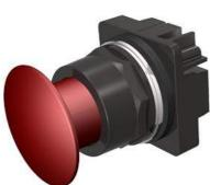
30mm BlackMax, Epoxy Coated Corrosion Resistant Metal Operator, Round Push-Pull Operator Non-Illuminated Mushroom Head Cap Small 1.73" (44 mm) Metal, Anodized Red 3 Position Pull-Momentary/Push-Maintained UL Listed, CSA Certified NEMA 1,3,3R,4,4X,12,13 & Automotive Standards
