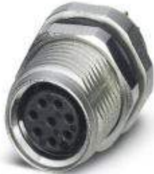
Sensor/actuator flush-type plug-in connector, socket, 8-pos. M8, rear/screw mounting with M10 fastening thread, with straight solder connection
