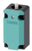
Position switch basic switch plastic 40 mm, according to EN 50041 Increased corrosion protection Device connection 1 x (M20 x 1.5) 1 NO/2 NC quick action contacts functional at -40 °C Shock and vibration test according to EN 61373, Category 1B
