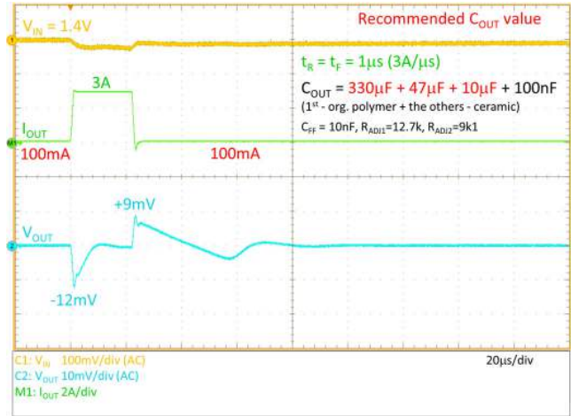
Figure 77. Load Transient Response, ADJ-0.5V set to 1.2V
