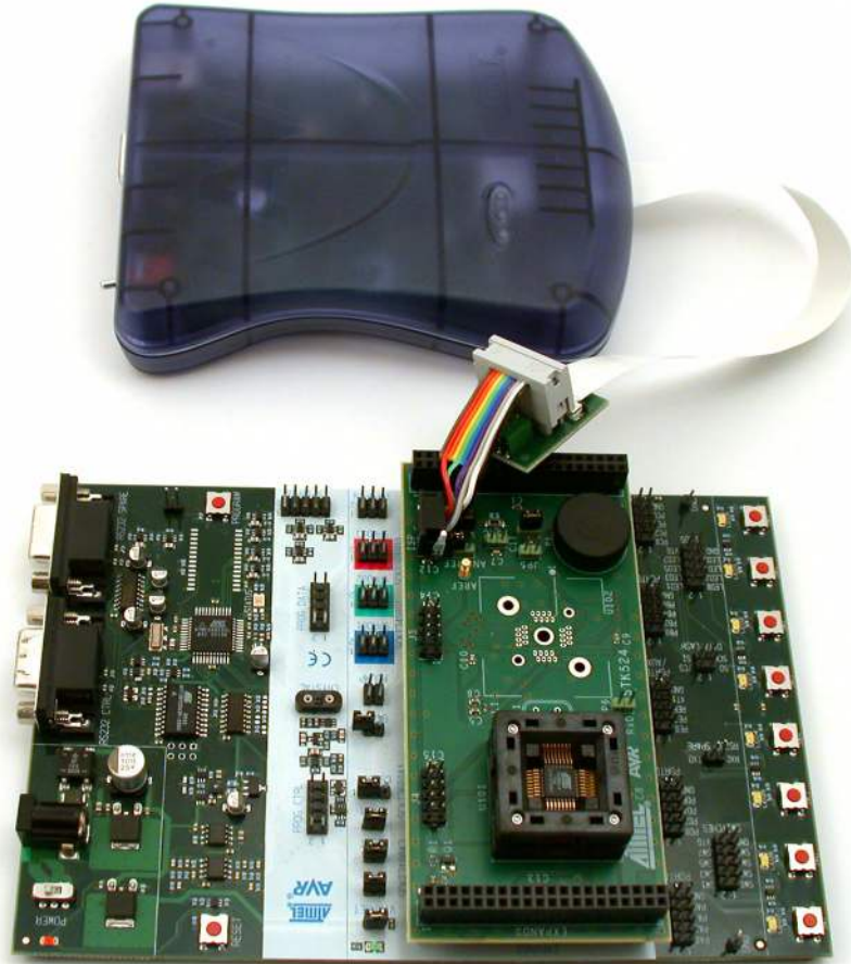
Figure 4-3. Connecting JTAGICE mkII to the STK524
