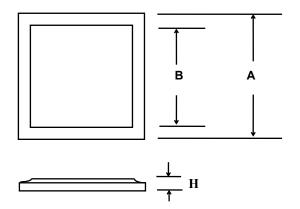
Bottom side metallization Ag thickness is 5KA minimum Top side metallization Al thickness is 25KA minimum Bottom side is cathode, top side is anode Dimension H =0.0105±0.001(0.27±0.026) (It can be customized according to customer requirements)
