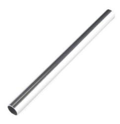
**Description:** These 8" long aluminum tubes have an outer diameter of 5/8", an inner diameter of 0.569", and a wall thickness of 0.028". When used with the mating tube clamps, these can be used for versatile structural support. Additionally, wires and cables can easily be run through the center.
