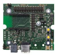
The power to deRFnode and deRFgateway is either supplied by USB, an AC adapter or 3xAA batteries. As programming interface, the standard JTAG connections for ARM and AVR are present together with other standard interfaces like SPI, UART and I2C. Additional sensors for special measurement tasks can be connected using the 34 pin expansion header.
