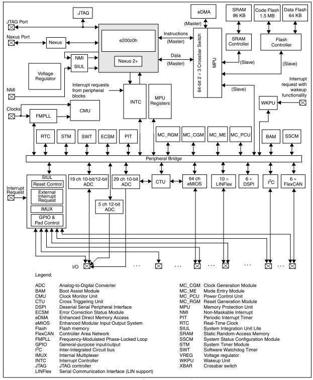
Figure 1. MPC5607B block diagram
