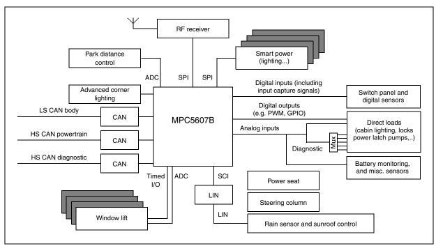
Figure 2. Body controller application example
