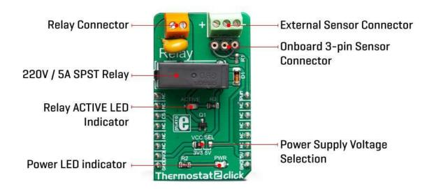
The 1-Wire® communication with the host MCU is performed over the PWM pin of the mikroBUS™. Depending on the temperature information obtained over the 1-Wire® interface, the host MCU can take the necessary action: it can either open or close contacts of the relay.
