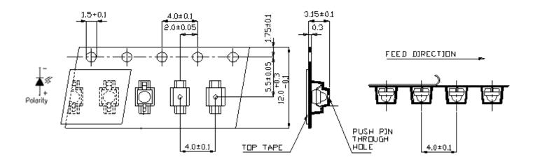
Note: The tolerances unless mentioned are ±0.1, unit=mm.
