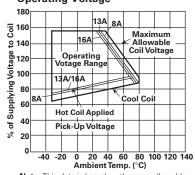
**Note:** This data is based on the max. allowable temperature for E type insulation coil (115°C).
