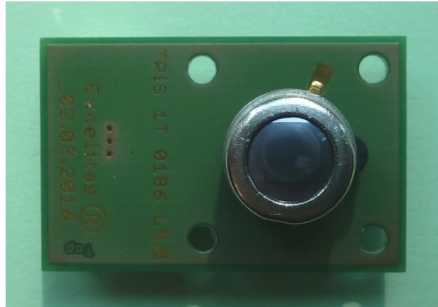
Figure 9: Alignment of TO housing nose with the marking on the board.
