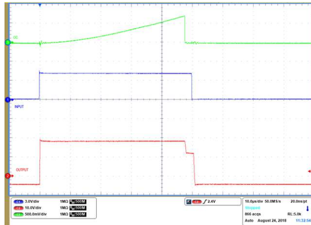
Figure 13. Expanded Short Circuit Waveforms for UCC21710
