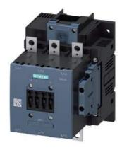
power contactor, AC-3 150 A, 75 kW / 400 V AC (50-60 Hz) / DC operation 500-550 V AC/DC auxiliary contacts 2 NO + 2 NC 3-pole, frame size S6 busbar connections drive: conventional screw terminal
