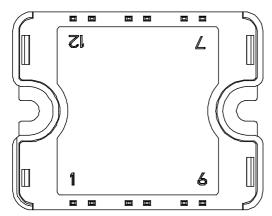
All multiple inputs and outputs must be shorted together 3/4; 5/6; 7/8; 1/2; 9/10
