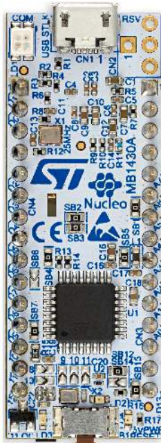
NUCLEO-G431KB example. Boards with different references show different layouts. Picture is not contractual.
