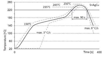
Resistance to soldering heat - reflow profile IEC 60068-2-58
