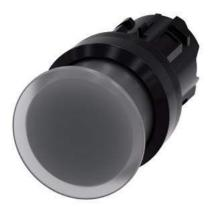
Illuminated mushroom pushbutton, 22 mm, round, plastic, clear, 30 mm, momentary contact type, with laser labeling, symbol number according to, ISO 7000 or IEC 60417
