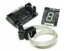
This shiftout LED Kit includes a very simple and small LED display module. It makes it possible for you to directly connect many 7-segment led modules in a chain. So you could diy a simple timer or a clock display , and many other devices that require the use of 7 segment LEDs.
