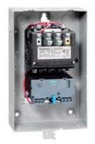
Non-reversing motor starter Size 1 Three phase full voltage Solid-state overload relay OLRelay amp range 3-12A 550/575-600 50/60HZ coil Combination type Indoor general purpose use
