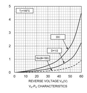
REVERSE POWER DISSIPATION:P<sub>R</sub>(W)
