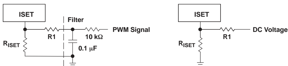
Figure 10. Analog Dimming Using an External Voltage Source to Control the Output Current
