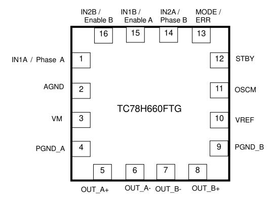
Note: Please solder the corner pads and the rear thermal pad of the QFN package, to the GND pattern of the PCB.
