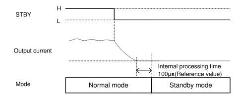
If the output current is zero-detected, the operation mode enters into the standby mode after 100 $\mu$ s. The mode enters into the standby mode forcedly after 1 ms(max) from STBY=L.
