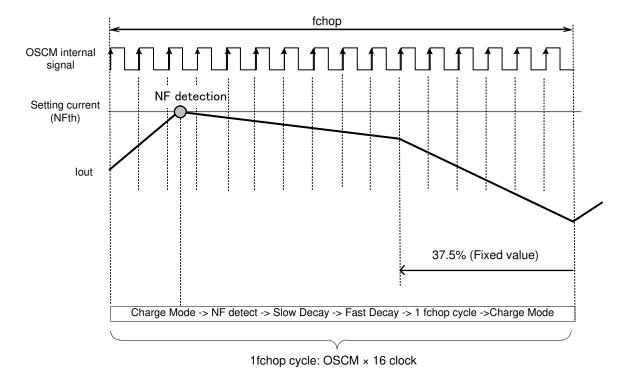
Note: The blanking time(AtBLK) is also set to prevent an incorrect operation in the NF detection (the motor current reaches the set current value (NFth)).
