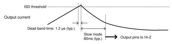
Note: Above ISD operation threshold value and band times are reference values, and are not guaranteed.
