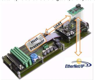
Software integration with a Host processor is also easy since no re-programming is required on the Host processor and the Host firmware is never touched. The *RapID Universal Gateway* conforms to the Host messages passed over the UART by using a "script". This script transforms the UART messages into the appropriate EtherNet/IP messages. Simply write a script to interpret the UART messages and the field device is ready to talk on the network.
