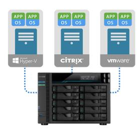
The Lockerstor 10 Pro provides enterprise-class hardware and software and is compatible with VMware, Citrix, Hyper-V virtual storage environments. iSCSI/IP-SAN and NFS support allow it to seamless integrate with existing IT environments, providing an optimal and cost-effective storage solution.
