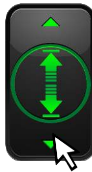
Manually drive head down until nozzle is approximately 2mm above SCS-LAT
