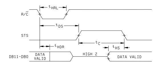
LOW PULSE FOR R /  $\overline{C}\,$  - OUTPUTS ENABLED AFTER CONVERSION
