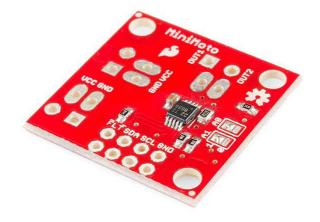
SparkFun's MiniMoto board is an I<sup>2</sup>C-based DC motor driver. It's designed to be used in a system with up to 8 additional MiniMotos, all on the same data lines.
