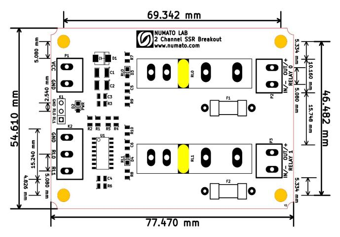
L x W x H : 77.470 mm x 54.610 mm x 30 mm Mechanical Hole Diameter- 4.0 mm
