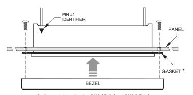
\*Sealing gasket is optional on DMS-BZL2-C and DMS-BZL4-C
