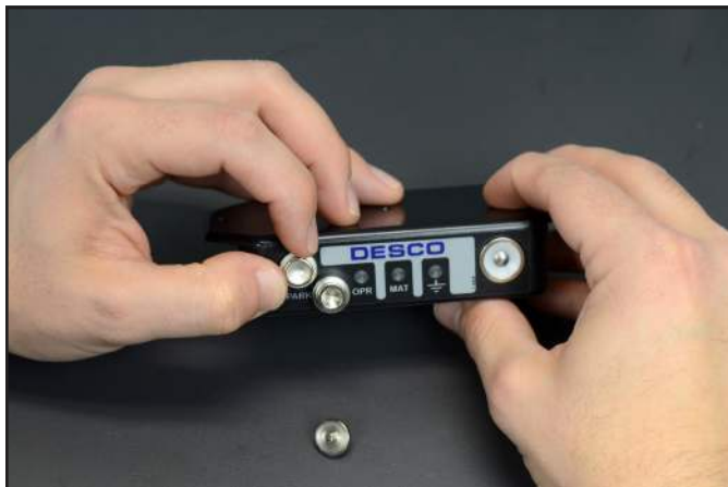
Figure 12. Installing the 10 mm snap adapters to the 19322 Full-Time Continuous Monitor
