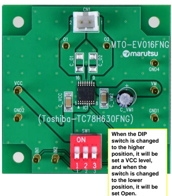
This evaluation board has a DIP switch (SW) so that the operation setting of the TC78H630FNG can be set without the external signal input.
