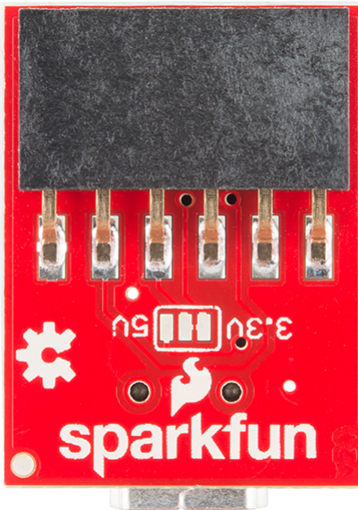
6 pin SIL, 0.1" pitch header at top of PCBA
