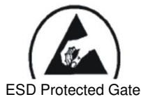
ESD Protected Gate
