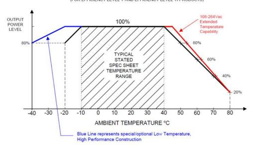
+74C operation with an output power of 19.2W; and cold start at -40C
