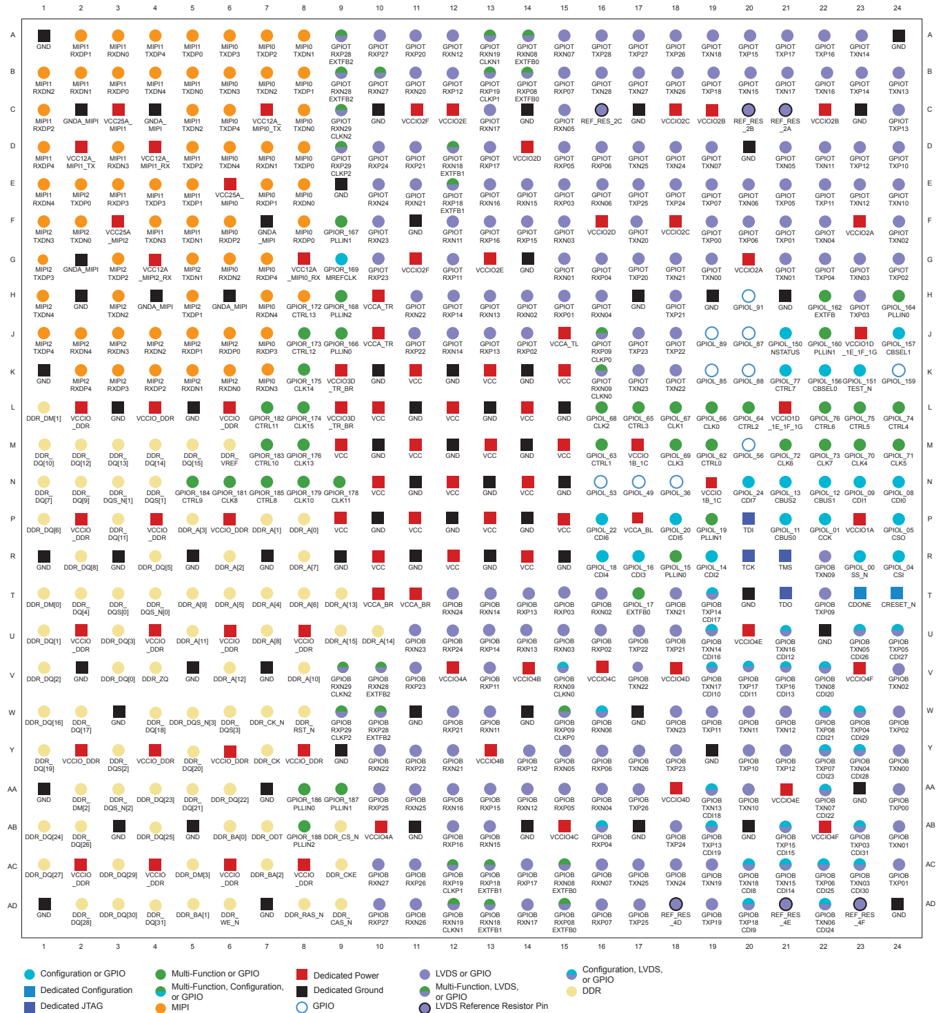
Figure 39: 576-Ball FBGA Pinout Diagram
