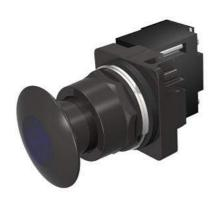
30mm BlackMax, Epoxy Coated Corrosion Resistant Complete Metal Unit Illuminated Push-Pull Operator Transformer type, 240V AC LED Lamp Mushroom Head Cap Small 1 3/4" (44.5 mm) Metal, Black with Blue Lens 2 Position Maintained, Pull-to-Release UL Listed, CSA Certified NEMA 1,3,3R,4,4X,12,13 & Automotive Standards
