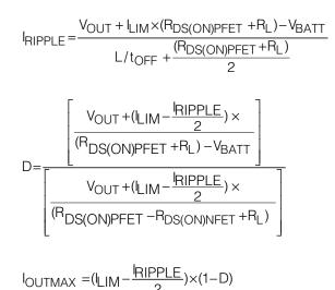
Here,  $I_{LIM}$  is the NFET current limit (800mA typ), toFF is the LX switch's off-time (0.25 $\mu$ s typ), and RL is the series resistance of the inductor.
