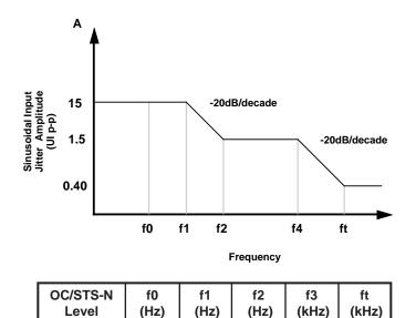
Figure 1. Input Jitter Tolerance
