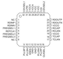
32-Pin EPAD TQFP (H32-1)
