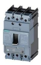
circuit breaker 3VA5 UL frame 125 breaking capacity class S 25kA @ 480 V 3-pole, line protection TM240, ATAM, In=100A overload protection Ir=80A ...100A short-circuit protection Ii=5...10 x In cable connection on both sides
