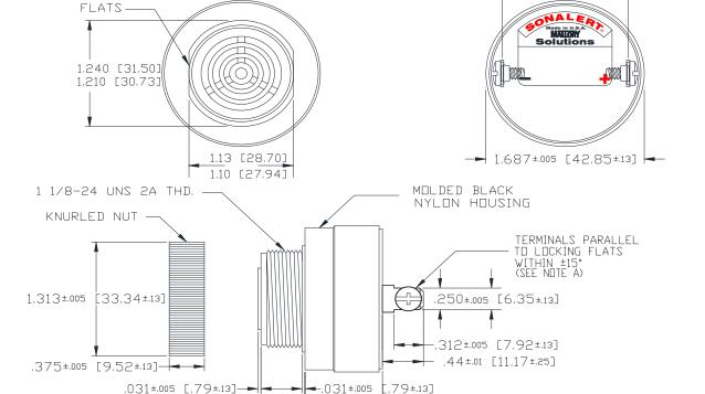
NOTE A: TERMINALS-.032 BRASS TIN PLATED, TAPPED FOR #6-32 SCREW. TWO #6-32 NICKEL PLATED BRASS SCREWS INCLUDED. WILL ACCEPT 1/4" QUICK CONNECT.
