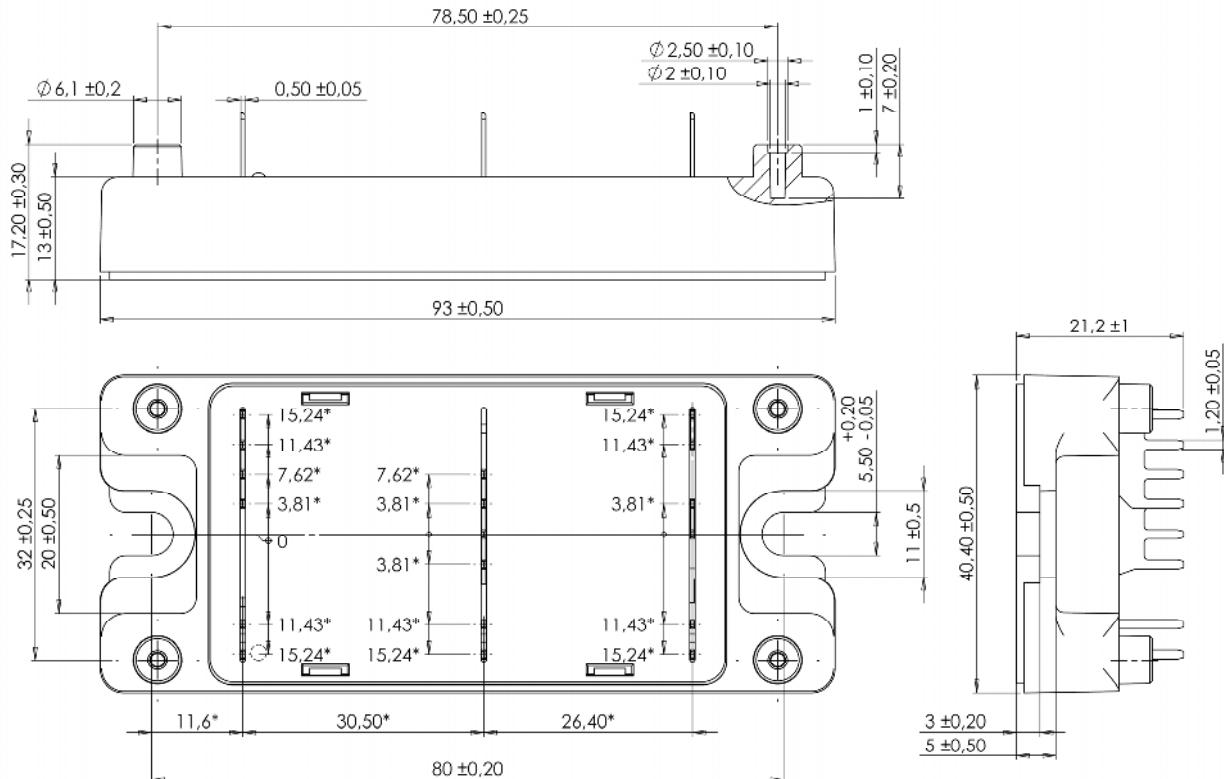
ALL DIMENSIONS MARKED "\*" ARE TOLERANCED AS  $\pm 0.10$  mm
