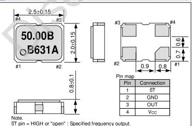
ST pin = LOW: Output is high impedance, oscillation stops.
