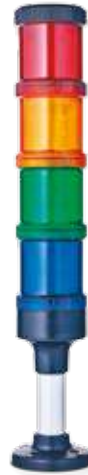
Order number: ECO60-Q05 Colours: red/orange/green/blue Function: LED steady beacon Nominal voltage: 24 V AC/DC Type of mounting: Tube mounting (100 mm tube length)
